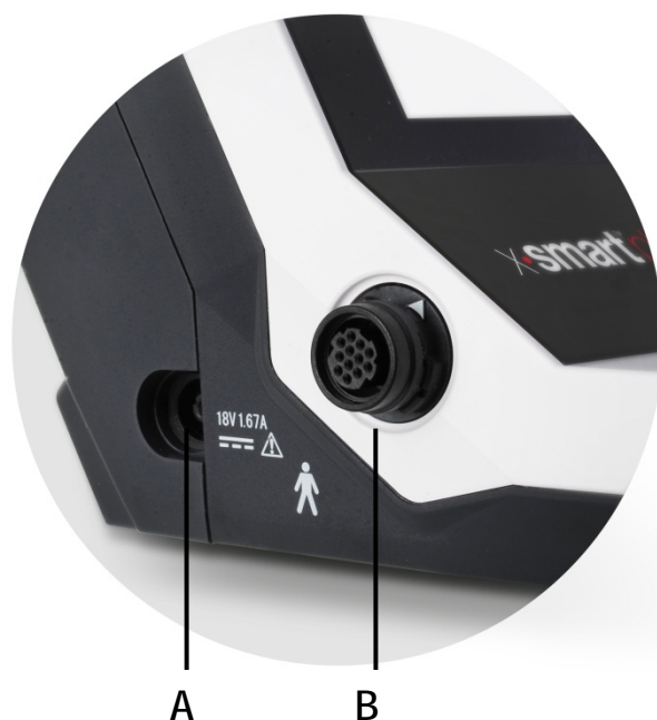
Fig. 4 Power and Motor handpiece connectors
